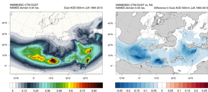
Difference in JJA mean Mineral dust AOD at 550 nm from NMMB/BSC-CTM 1994-2013 Radiatively active vs. non-radiatively active
